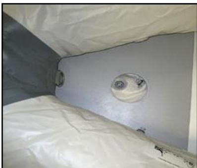
Install rear aluminum panel, make sure it fits under the height board located on the transom
